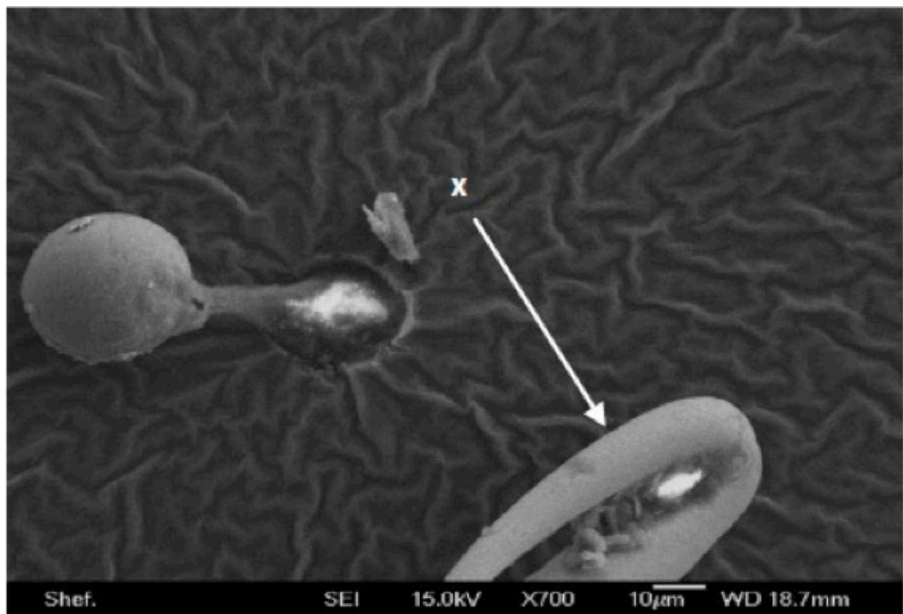
Fig. 4: Nanomanipulator needle (X) returned to foreground after removing the large spherical object from its impact resting place, showing impact site and material issuing from the LSO.
